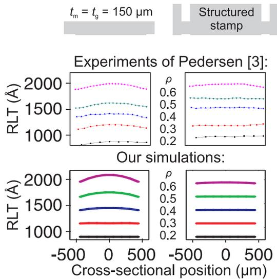
**Fig. 3** A structured stamp with narrow flexures separating thicker feature-carrying mesas reduces systematic RLT variation.  $\rho$ : protrusion density. Resist viscosity fit:  $2 \times 10^5$  Pa.s.  $t_m = 525 \mu m$ ;  $t_g = 150 \mu m$ ;  $s_m = 1.5$  mm;  $g = 500 \mu m$ . Stamp-average pressure: 0.35 MPa; imprint time: 5 min.
