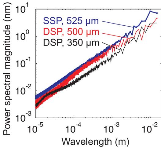
**Fig. 1** Power spectra of the topographies of three different virgin silicon wafers: single-side-polished (SSP), 525 μm thick; double-side-polished (DSP) 500 μm thick; DSP 350 μm thick. Wavelengths up to approx. 13 nm are shown.
