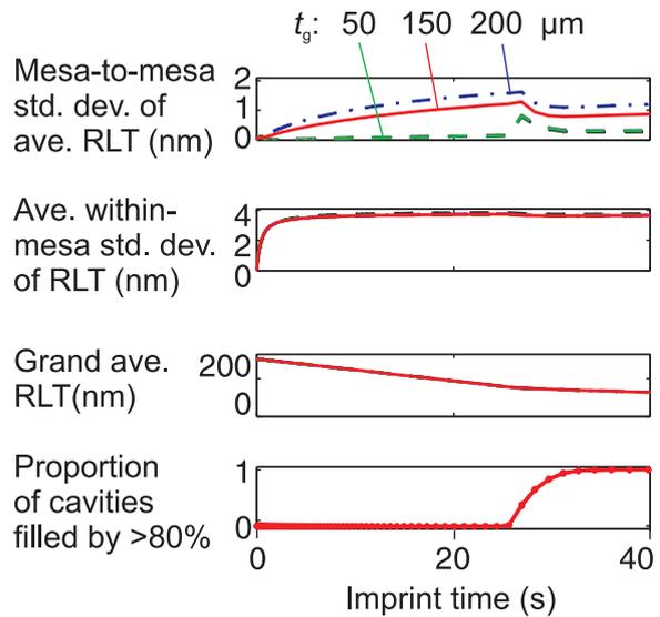
**Fig. 4** Simulations of imprinting a  $5 \times 5$  array of mesas into a 7.5 mm-square region. Measured wafer nanotopography (525 μm SSP wafer) was fed into simulation. Random mesa-to-mesa RLT variation reduces with smaller  $t_g$ , while systematic within-chip variation is relatively insensitive to  $t_g$ . Process as Fig. 3;  $\rho = 0.3$ .
