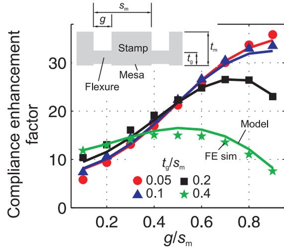
**Fig. 2** Stamp compliance is considerably increased by the presence of backside grooves. ‘Compliance enhancement factor’ is the ratio of pk-pk deflection of the structured stamp to that of a uniformly  $t_m$ -thick stamp, under identical loadings. Symbols: finite-element simulations; lines: semi-analytical model. Inset: stamp cross-section.  $t_m/t_g = 3.3$ .
