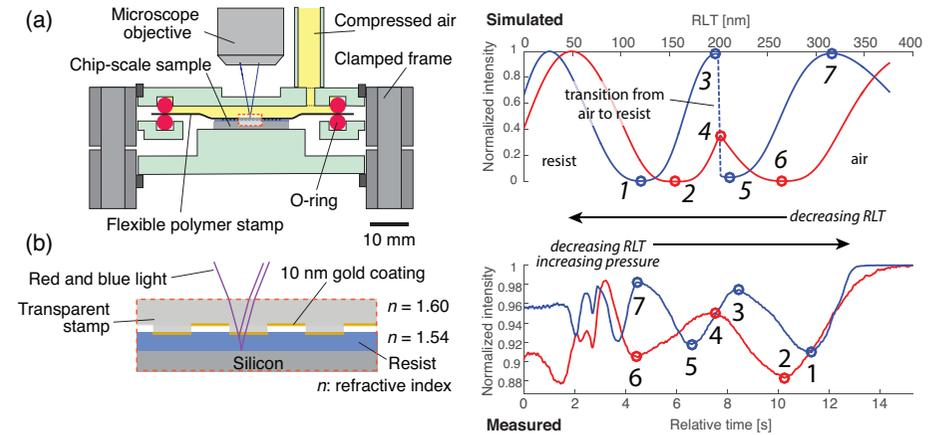
Figure 1. (a) Cross-section of the testbed [5]. A back-pressurized stamp contacts a deformable resist layer, while an objective relays the reflected light field to a CMOS sensor (not shown). (b) Section view of the stamp-resist contact region.
