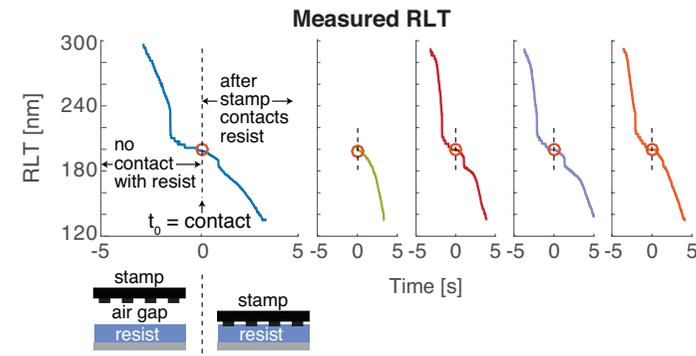
Figure 3. RLT values are assigned to time points in the experiment by matching a point's measured normalized intensity to the simulated intensity. For each time point the color channel offering the higher RLT sensitivity at that point is used. Each trace corresponds to a different resist region in the same video.
