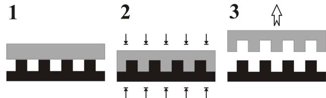
Fig. 1 Process schematic for thermoplastic imprinting, or hot micro-embossing
