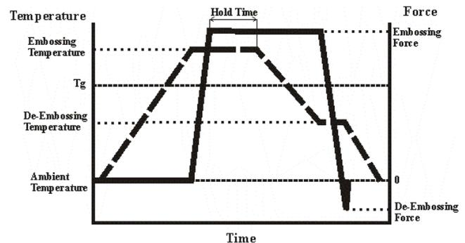
Fig. 2 Process parameters for typical thermoplastic imprinting, or hot micro-embossing.  $T_g$ =Glass transition temperature
