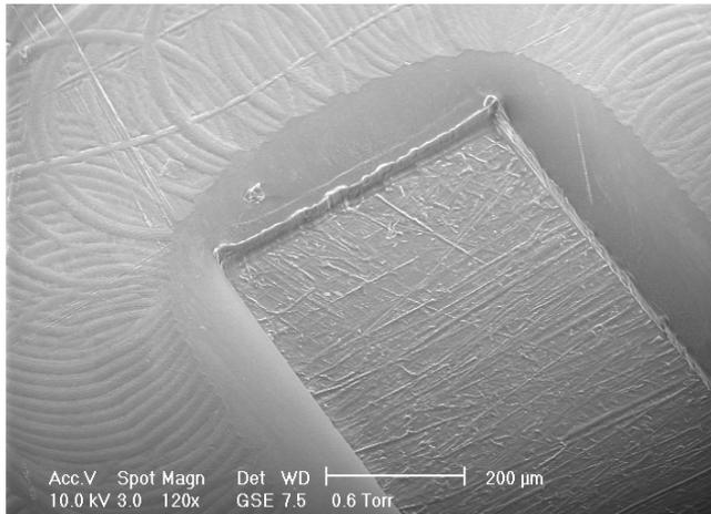
*Fig. 4 Oblique SEM micrograph of PMMA embossed with a machined copper tool, reprinted from [22]. Note the replicated machining marks.*
