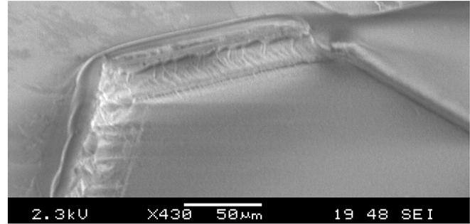
*Fig. 3 Oblique SEM micrograph of a hexagonal feature on a PMMA part embossed with a silicon tool. The part was formed at 120°C under 0.6 MPa maintained for 3 min. The tool and part were separated at 50°C. The severe distortion of the left edge of the feature is attributed to thermal contraction. The edge of the part is toward the upper left. This image has been lightened and cropped from the original.*
